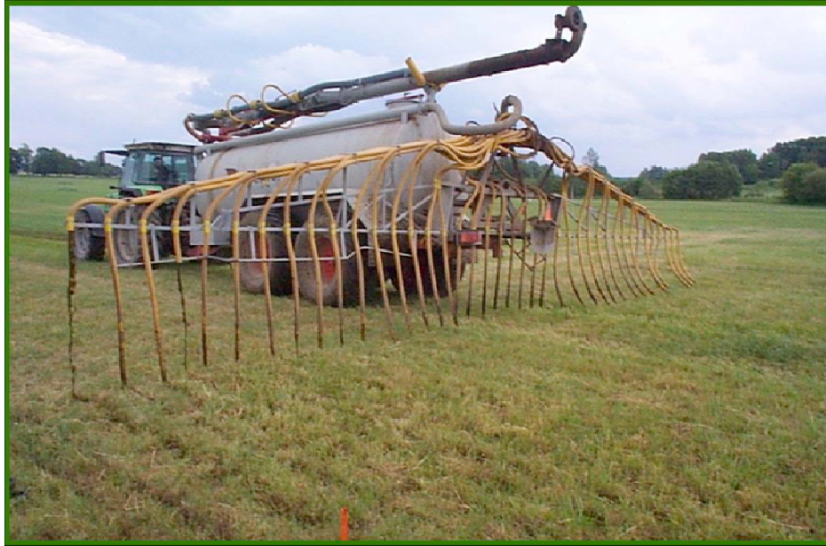
Figure 1. Spreading of digestion residues with a trailing hose spreader. Photo: Lena Rhode.
