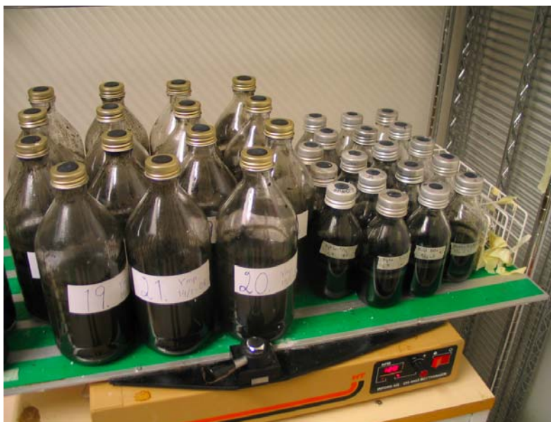
Figure 2. Batch digestion test. The bottles are sitting on an oscillating table. Photo: Anna Schnürer.
