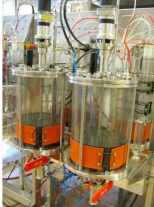
Figure 4. Continuous biogas reactors at laboratory scale (8 L). Photo: Anna Schnürer.
