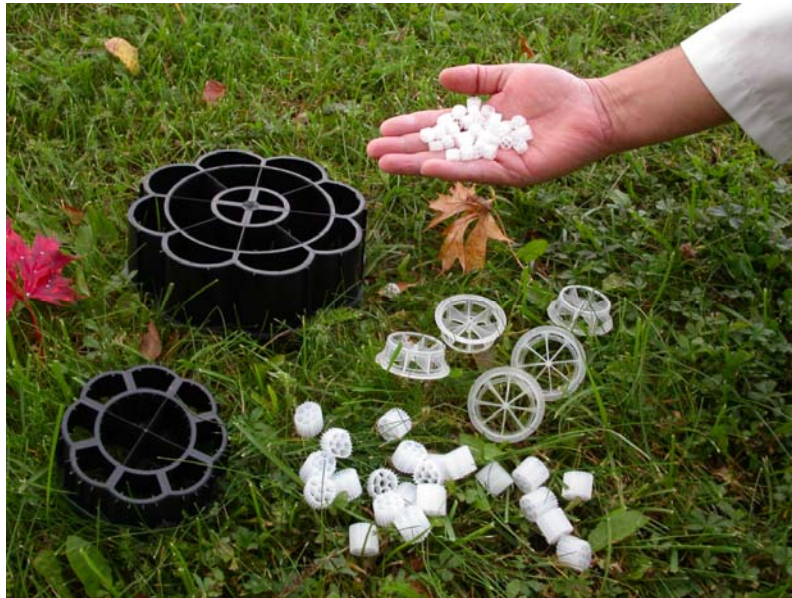
Figure 7. The plastic rings can be used as carrier material in anaerobic filters. Photo: Åsa Jarvis.
